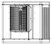
Proceed with the installation as normal. The Side Sealer Channels will go on the same flanges as for a horizontal duct. You may use the Side Sealers provided to close off the window above your cooler's duct.
