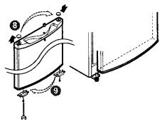
Reassemble the refrigerator door stopper  ${\rm (I)}$
