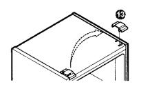
**12** Assemble the upper hinge  $\boldsymbol{0}$  and the cap  $\boldsymbol{0}$ .
