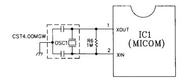
This circuit generate the base clock for calculating time and the synchro clock for transmitting data from and to the inside logic elements of the IC1(MICOM). Be sure to use the exact replacements parts since the calculating time by the IC1 may be changed or it will not work if the OSC1 SPEC is changed.
