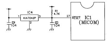
The RESET circuit is for allowing all the functions to start at the initial conditions by initializing various parts including the RAM inside the MICOM (IC1) when the power is initially supplied or the power supply to the MICOM is restored after a momentary power failure. For the initial 10ms of power supply, LOW voltage is applied to the MICOM RESET terminal. During a normal operation, 5V is applied to the RESET terminal. (If trouble occurs in the RESET IC, the MICOM will not work.)
