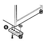
**8** Move the cap **(b)** and reassemble the center hinge **(b)** after removing the washer.
