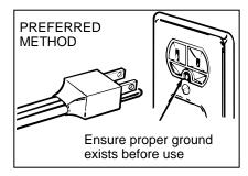
This appliance is equipped with a cord having an equipment grounding conductor and a grounding plug. The plug must be plugged into an appropriate outlet that is properly installed and grounded in accordance with local codes and ordinances.
