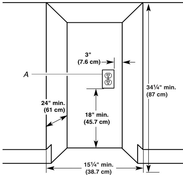
A. Grounded electrical outlet must be a minimum of 3" (7.6 cm) away from surrounding cabinets or nearby walls as shown. It can be placed either to the left or the right side of the product.
