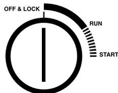
**NOTE:** When the compacting cycle is done, turn the Key-Knob to OFF & LOCK. Remove the Key-Knob and store it out of children's reach.
