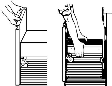
4. Place the other 2 corner posts on the floor to the side of the compactor. Grasp the sides of the compactor cabinet and put compactor on its side on top of the corner posts. Remove the shipping base from the bottom of the compactor.
