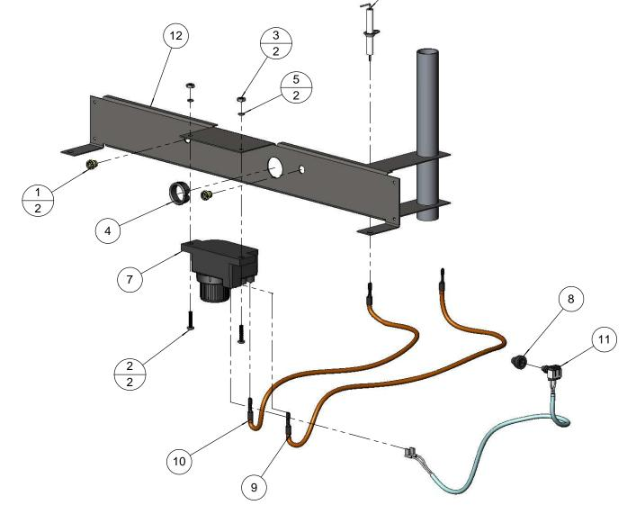
**NOTE:** ITEM 12 (ASSEMBLY 510-0398) IS SHOWN FOR ILLUSTRATION AND GENERAL ASSEMBLY PURPOSES ONLY. THIS ASSEMBLY IS ACTUALLY PART OF THE MAIN BODY ASSEMBLY 510-0378 SHOWN ON DRAWING 500-0063B
