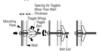
Place the mounting plate against the wall and insert the toggle wings into the holes in the wall to mount the plate.
