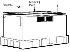
**5** Remove the 2 screws from the mounting plate. This plate will be used as the rear wall template and for mounting. You may discard these screws.
