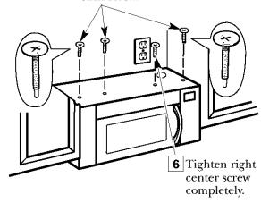
7 Tighten the remaining three screws to the top of the microwave oven. (While tightening screws, hold the microwave oven in place against the wall and the top cabinet.)
