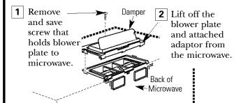
3 Slide exhaust adaptor to one side and remove it. **NOTE:** The exhaust adaptor with damper is not needed for recirculating models. You may want to save them for possible future use.
