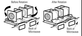
Gently remove the wires from the grooves.
