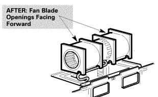
**NOTE:** Make sure wires remain routed in the grooves of the motor frame.
