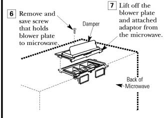
8 Slide exhaust adaptor to one side and remove it.
