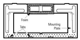
Attach the other 28" foam tape to the front of the mounting plate around both of the exhaust openings where it will touch the microwave.
