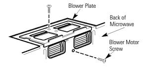
**8** Replace the blower plate in the same position as before with the screw.
