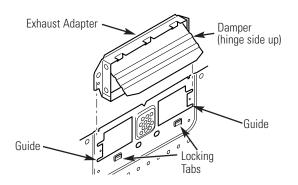
Push in securely until it is in the lower locking tabs. Take care to assure the damper hinge is installed so that it is at the top and that the damper swings freely.
