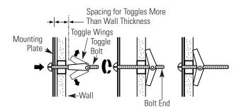
Place the mounting plate against the wall and insert the toggle wings into the holes in the wall to mount the plate.
