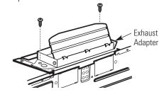
Attach the exhaust adapter to the oven rear panel by sliding it into the guides at the top center of the back of the oven.
