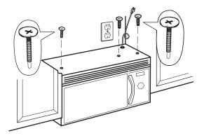
Tighten the three screws to the top of the oven completely. (While tightening screws, hold the oven in place against the wall and the top cabinet.)
