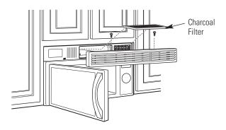
Insert the filter into the top of the opening, between the side support slots.
