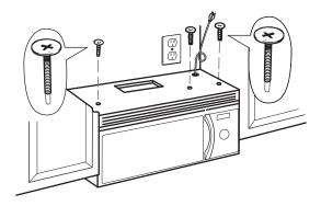
Tighten the three screws to the top of the oven completely. (While tightening screws, hold the oven in place against the wall and the top cabinet.)
