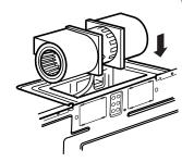
Replace blower plate and replace screws for blower plate and blower motor removed in Step 1.
