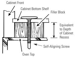
Attach the oven to the top cabinet by inserting 3 self-aligning screws through outer top cabinet holes. Turn two full turns on each screw. Be sure to keep power cord tight. Be careful not to pinch the cord, especially when mounting flush to bottom of cabinet.
