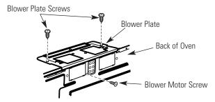
2 Slide the blower plate from under its retaining flange and lift it off.
