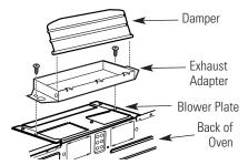
**NOTE:** On some models, the exhaust adapter and damper assembly may already be assembled to the oven.
