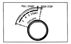
To get the full benefit of the Delicate Cycle, always set it at the beginning of the cycle. During wash, the Delicate Cycle alternates between agitation and pauses to protect delicate clothes.
