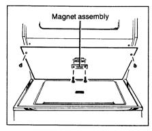
Take out 2 screws holding the magnet assembly and remove the magnet assembly.
