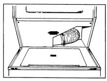
The washer lid can now be opened enough to allow you to remove the agitator, and the dryer exhaust ducting is accessible for inspection and cleaning.
