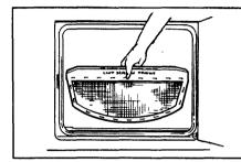
Remove the lint filter by pulling straight out. Wipe all accumulated lint from screen. Occasionally wash filter using soap and warm water. Rub lightly, rinse and dry thoroughly. This will help remove all fabric softener buildup.
