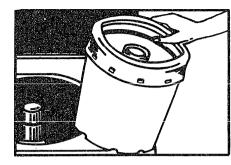
• Place Mini-Basket tub on agitator. Pull the agitator toward the front of the machine for easier installation and removal of Mini-Basket tub.
