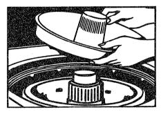
• After loading clothes in the Mini-Basket tub, *be sure to replace the Filter-Flo pan*. The pan serves as a lid to keep the clothes in the Mini-Basket tub. • Put <sup>1</sup>/<sub>4</sub> to <sup>1</sup>/<sub>3</sub> cup (60 to 80 ml) detergent in Filter-Flo pan.
