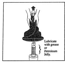
The Activator® agitator. Remove at regular intervals—about 4 to 6 months—and remove any lint that may have accumulated. No tools are needed, simply grasp agitator with both hands and pull straight up sharply. The slotted section at the top of the metal shaft has a light coating of lubricant to prevent parts sticking together. If this area appears to be dry, apply a light coat of grease or petroleum jelly around the slotted section of the shaft before replacing the agitator. Do not overgrease.
