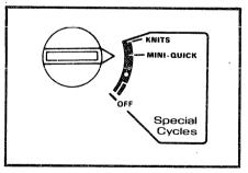
• Pull Cycle Selector Knob to start washer. Cycle will be completed automatically.
