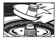
• After loading clothes in the Mini-Basket tub, *be sure to replace the Filter-Flo pan*. The pan serves as a lid to keep the clothes in the Mini-Basket tub.
