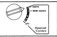
MINI-QUICK CYCLE— For small, lightly soiled loads you need in a hurry. Use with MINI-BASKET tub only.
