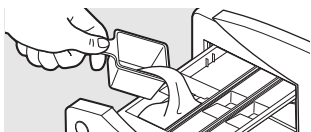
Insert in forward position for liquid detergent
