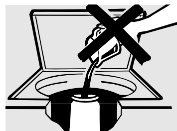
Do not pour anything into the agitator if the top is removed
