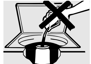
Do not pour anything into the agitator if the top is removed
