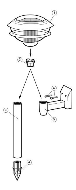
A flathead screwdriver is required for mounting the wall bracket.
