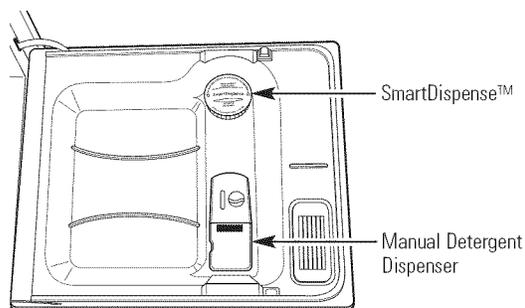
The cover of the manual dispenser will open during the wash cycle. If you are using SmartDispense™, leave the cover of the manual dispenser open before starting the cycle.
