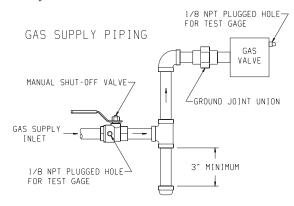
Figure 2 - Method of Installing a Tee Fitting Sediment Trap
