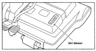
The lights give you an indication of the amount of dirt particles that are passing thru the sensor on its way to the dust bag.
