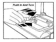
2. Push in and turn bulb counterclockwise to remove.
