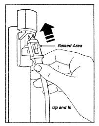
2. Connect POWER-MATE™ plug and cord as shown. DO NOT force. Raised area of plug must be toward hand.
