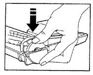
3. Snap brush supports into place on base. Be sure brush supports are not upside-down. 4. Line up front of cover and base. Rest cover on front edge of base as shown.
