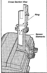
the illustration a dirt sensor element is located on the Inside of the swivel. approximately three and a half inches down. Note the arrows. Each element should be cleaned periodically. To reach the sensor elements, use a small brush such as a bottle brush. Brush each sensor element several times to remove dust and dirt.
