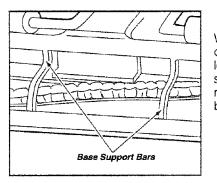
When brushes are worn to the level of the base support bars, replace the brushes.
