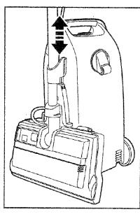
The lower wand has a "U" shaped flange in the area where the power cord attaches. The base has a "U" shaped slot near the front caster.
