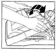
6. Tilt cover to back. Press cover firmly until side tabs snap into place. Replace cover screws, light bulb and light cover.
