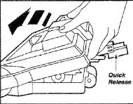
4. Turn POWER-MATE™ right side up. Press handle release pedal and lower the swivel. Tilt cover forward from back until front snaps free.
