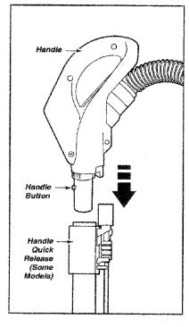
2. Insert handle into wand until lock button snaps in place. Be sure hose is not twisted.
