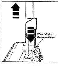
2. Press wand release pedal with foot and pull the wands straight up out of POWER-MATE<sup>TM</sup>.
