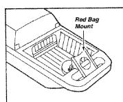
red bag mount. 5. Check and clean motor safety filter. The red bag mount will flip forward after removing bag. This will prevent the lid from closing until a new bag is installed.
