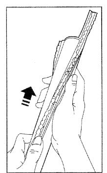
5. Reassemble brush assembly. To line up screw holes in dowel, sprocket and end brush, be sure beater bar portion of end brush lines up with beater bar on brush dowel.
