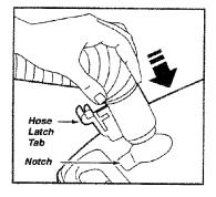
1. Line up the hose latch tab and notch in canister hood and insert hose into canister until it snaps in place.
