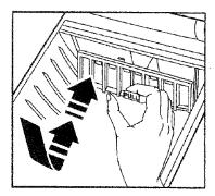
4. Snap filter back into canister.
