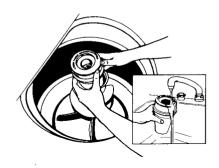
5. Clean dispenser after each use with warm water. To remove the dispenser, grasp the top of the dispenser with both hands. Squeeze and push upward with thumbs to remove. Clean by holding under water faucet. Replace after cleaning.
