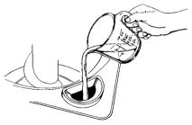
3. Start the washer. Bleach will be diluted automatically during the wash part of the cycle.
