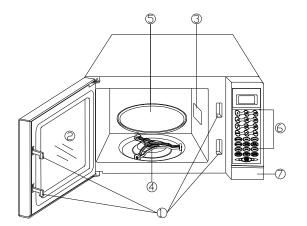
Door Safety Lock System Oven Window Wave Guide Turntable roller Glass Tray Control Panel Door Release Button
