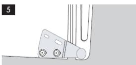
Remove the two screws from top bracket and replace on the other side. You will need to first remove the plastic caps from the other side.
