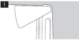
Remove the plastic covering from the bottom door hinge.
