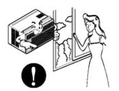
If water enters the product, turn off the the power switch of the main body of appliance. Contact service center after taking the power-plug out from the socket.
