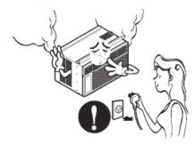
Do not use the socket if it is loose or damaged.
