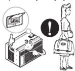
Do not place heavy object on the power cord and take care so that the cord should not be pressed.
