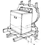
An Exhaust Hood should cap the exhaust duct to prevent exhausted air returning into dryer. The outlet of the hood must be at least 12 inches from the ground or anything else that may be in the path of the exhaust.
