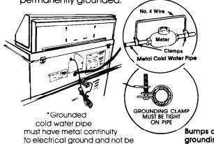
to electrical ground and not be interrupted by plastic, rubber or other electrically insulating connectors (including water meter or pump) without adding a jumper wire at these connections.
