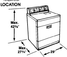
**Size:** Must be large enough to fully open dryer door. For recessed or closet installation spacing see back cover.
