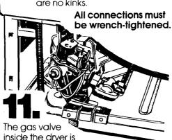
inside the dryer is shipped in the "ON" position. Check that the gas valve shut - off control is still in the "ON" position.
