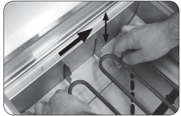
Fig. 18-1 Adjust cooking element
