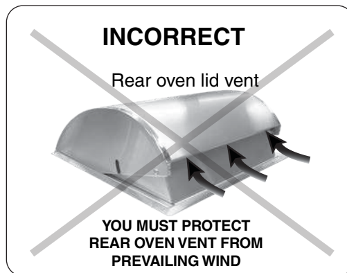
Fig. 8-3 Airflow direction - INCORRECT
