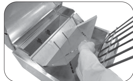
Fig. 22-4 Remove rear liner
