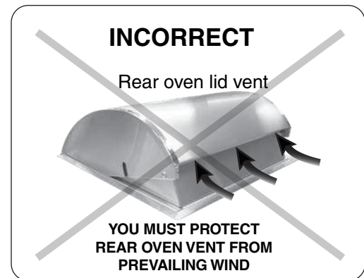
Fig. 8-3 Airflow direction - INCORRECT
