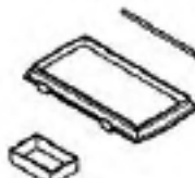
14844-1 DIRT CUP ASS'Y. (INCLUDES) 54492-1 DIRT CUP SUPPORT & LATCH ASS'Y. 14785-1 BAG FLANGE 55399-1 COVER PIN 01958-1 DIRT CUP 38289 GASKET 26265-2 CLAMP
