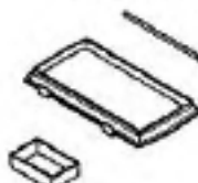
14844-1 DIRT CUP ASS'Y. (INCLUDES) 54492-1 DIRT CUP SUPPORT & LATCH ASS'Y. 14785-1 BAG FLANGE 55399-1 COVER PIN 01959-1 DIRT CUP 38289 GASKET 26265-2 CLAMP
