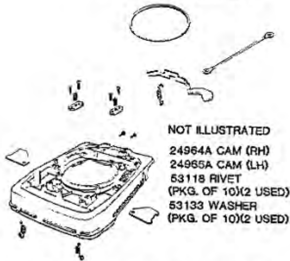
52334 FAN CHAMBER REPLACEMENT KIT (INCLUDES) 30517 MOTOR SEAL GASKET 13770-1 FAN CHAMBER COVER 53238-14 SCREW (PKG. OF 10)(2 USED)
