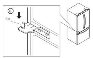
• Place the hinge in its original position (9) and place the two screws (10).
