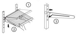
**NOTE:** Make sure that the shelf is installed in the horizontal manner. If not secured it can cause the shelves to fall, which will cause your stored food to spill.
