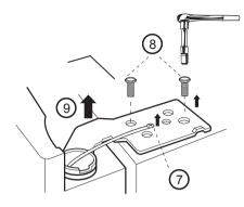
• Remove the door and place it over its inner face to avoid scratching.
