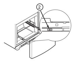
• With both hands, hold both sides of the door and pull up to separate it.
