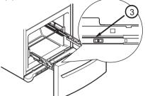
• With the drawer fully extended, insert the lower basket over the front part of the rail assembly and then the back part (4).
