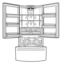
**Do not** block any of these vents with packages of food. This can interrupt the flow of air and cause temperature and moisture problems.
