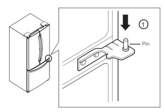
• Place the hinge in its original position (2) assembly the two pins (3) and the ground screw (4).
