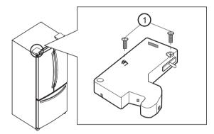
• With the 10 mm socket wrench, loose the two pins from the hinge (2) and remove it (3).
