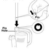
· To insert the upper piece of the metal handle, press on the pin that is on the upper handle and insert into the lower handle making sure that the pin comes out of the pinhole on the lower handle.
