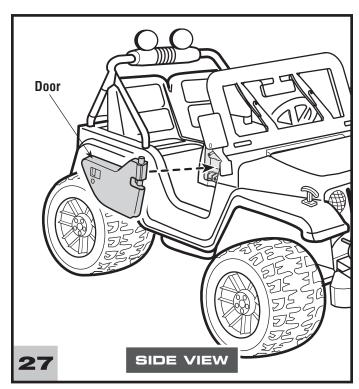
• Fit a door into the groove on the side of the dash. **Hint:** Each door is designed to fit one way. If the door does not fit, try the other door.
