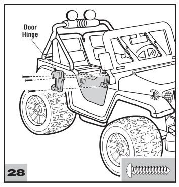
• Fit a hinge over the top end of the door.
