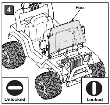
• Lower the hood on the vehicle. Using a slotted screwdriver, turn each lock fastener ¼ turn to the locked ● position.
