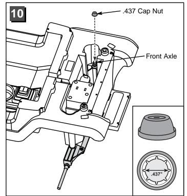
• Fit a .437 cap nut onto the end of each front axle.
