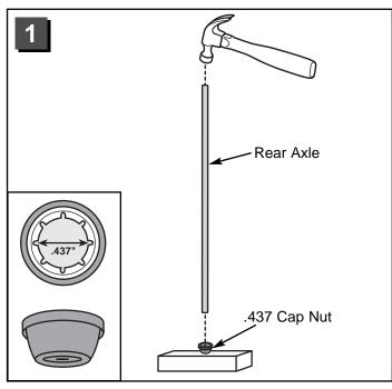
• Place a .437 cap nut on a flat surface, inside up, as shown. *Hint:* You may want to place a scrap block of wood underneath the cap nut to protect the assembly surface.
