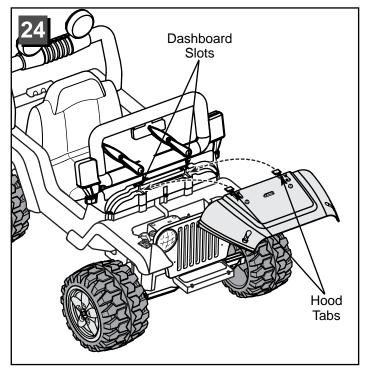
• Insert the tabs on the rear edge of the hood into the slots in the front of the dashboard.
