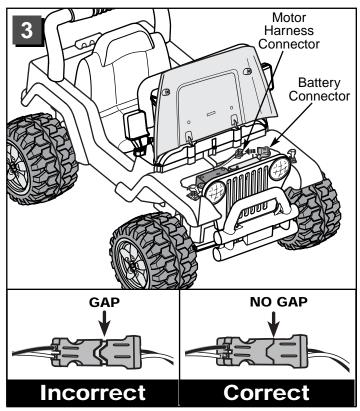
• Plug the battery connector into the motor harness connector.
