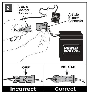
• Plug the battery connector and charger connector together. Push firmly to make sure the two connectors are completely joined.
