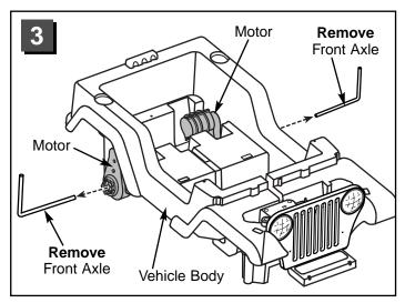
• Carefully remove the front axles from the motors in the vehicle body.
