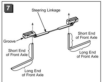
• Fit short end of the front axles up through the holes in the underside of the steering linkage. Make sure the long end of each front axle fits into the groove on each end of the steering linkage.
