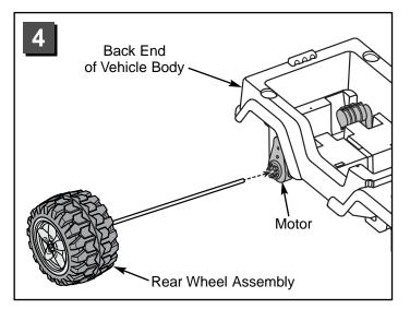
• Slide the rear wheel assembly through a motor and the back end of the vehicle body.
