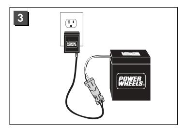
• Plug the charger into a standard 120 volt wall outlet.
