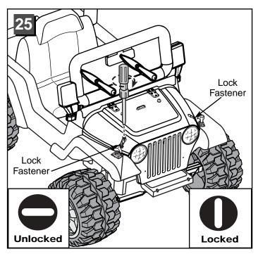
• Using a slotted screwdriver, turn each lock fastener in the hood 1/4 turn to the locked **①** position.
