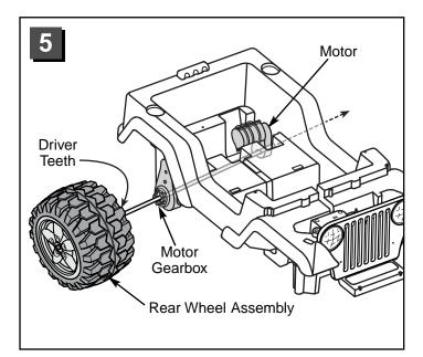
• Continue to slide the rear wheel assembly through the back end of the vehicle body, and out through the other motor.
