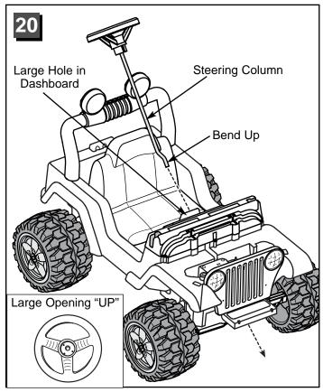
• Insert the steering column (with steering wheel) into the large hole in the dashboard. Make sure the large opening in the steering wheel and the bend in the steering column are facing UP.
