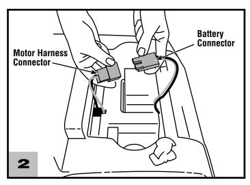
• Plug the battery connector into the motor harness connector. **Note:** If the battery connector will not plug into the motor harness connector, turn it over and try again. Do not force the battery connector into the motor harness connector.
