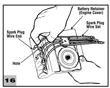
• "Snap" the ends of the spark plug wires set into the holes on the battery retainer (engine cover).
