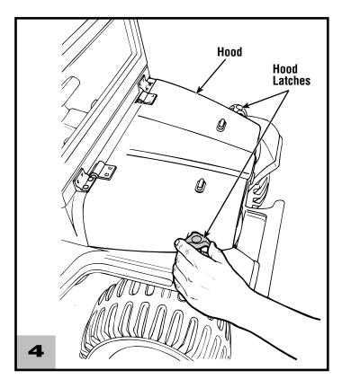
Lower the hood. Lift the hood latches and fit the short tabs onto the notches on the hood to secure it.
