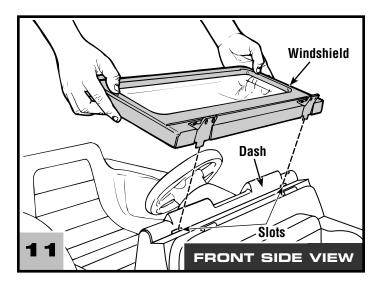
Fit the tabs on the back of the windshield into the slots in the top of the dash.
