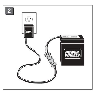
• Plug the charger into a standard 120 volt wall outlet. **Note:** If power flow to the wall outlet is controlled by a switch, make sure the switch is "ON".
