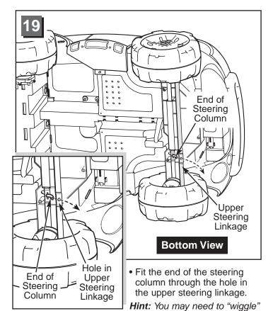
the end of the steering column to fit it into the hole in the 15 upper steering linkage.
