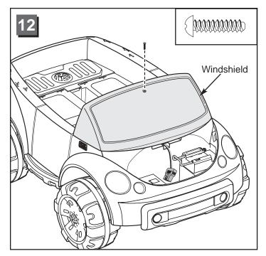
13 • Insert a #8 x  $^{3}/_{4}$ " screw through the hole in the top of the windshield. Tighten the screw.
