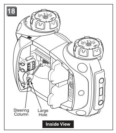
• Continue to slide the steering column up through the large hole in the dash.
