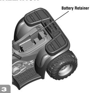
• Carefully lower the battery into the battery compartment. The battery retainer slides over the battery to secure it.
