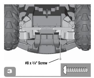
• Fit another #8 x <sup>3</sup>/4" screw through the hole shown in the front end and into the vehicle. Tighten the screw. *Hint:* You may need to adjust the front end to align the holes.
