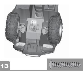
• Insert two #10 x 1" screws into the clip and tighten.
