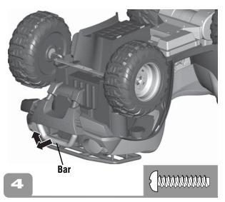
• Grasp the bar on the front end and pull it out and up to properly position the front end.
