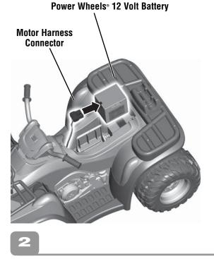
• Plug the motor harness connector into the battery.
