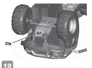
• Slide the clip (open side down) **under** the end of the steering column, as shown.
