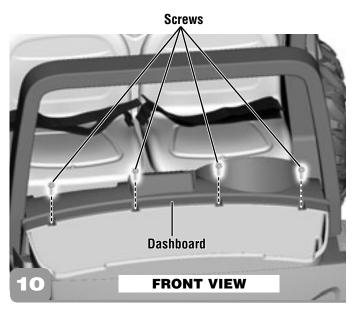
• Insert four screws through the dashboard and into the front end of the vehicle. Tighten the screws with a **short shaft Phillips screwdriver.**
