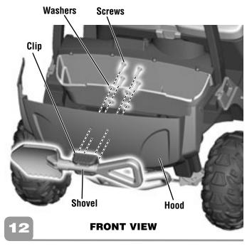
• Using safety scissors, carefully cut the plastic tie holding the shovel and clip together.
