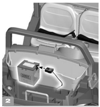
· Plug the motor harness connector into the battery.
