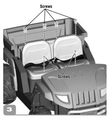
• Insert two screws into the seat area and four screws in the seat back. Tighten the screws.
