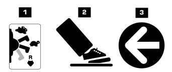
**IMPORTANT!** To avoid damaging the motors and gears, stop the vehicle before shifting from forward to reverse.
