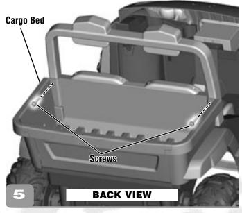
• Insert two screws through the cargo bed and into the ends of the sport bar. Tighten the screws.
