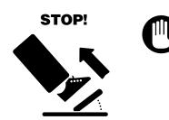
• Your vehicle has a patented, electronic braking system that automatically stops the vehicle when your child's foot lifts from the pedal. Make sure your child is comfortable with steering the vehicle and automatically knows how to stop.
