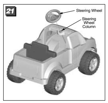
• Fit the steering wheel onto the end of the steering column and into the hole in the dashboard.
