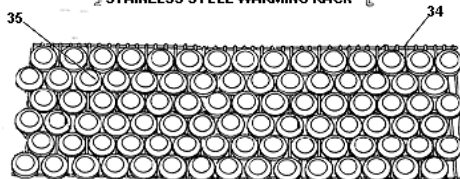
FOLLOW THIS PATTERN WHEN INSTALLING BRIQUETTES
