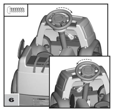
• While pushing down on the steering wheel, insert two #8 x 1/2" (1.3 cm) screws into the holes in the steering wheel base. Tighten the screws.
