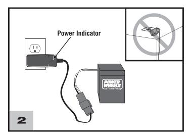
Plug the charger into a standard wall outlet.
