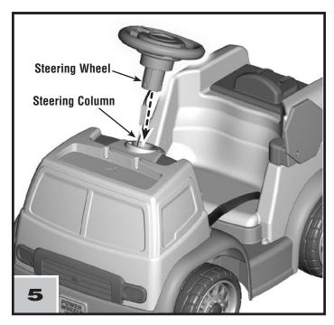
While carefully feeding the wire down into the dash, fit the steering wheel onto the end of the steering column.
