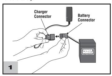
Plug the battery connector into the charger connector.
