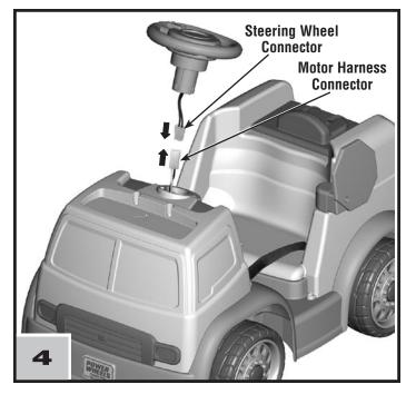
Plug the steering wheel connector into the motor harness connector.
