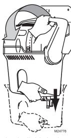
Use tap water to flush loose minerals from the tank. Sediment screen at tank's bottom is removable. For a more thorough cleaning, soak tank in warm, soapy water, then rinse clean. Tank is also dishwasher-safe.
