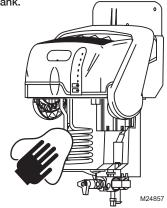
Once clean, reattach tank by securing the latch. Engage the water valve to the cam shaft, and "Lock" the shut-off valve. The "Press Reset" light will blink at start-up. Push the RESET button to ready the humidifier.
