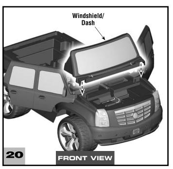
• Fit the tabs on the windshield/dash into the slots in the front end of the vehicle.
