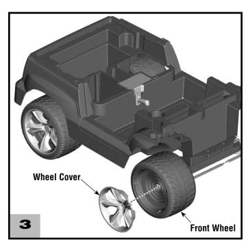
• Fit a wheel cover onto each front wheel.
