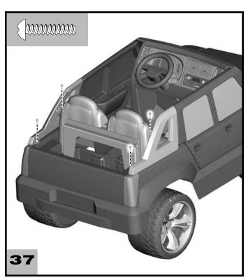
$\bullet$  Insert two #8 x  $^3/4^{\shortparallel}$  screws into each wing. Tighten the screws.
