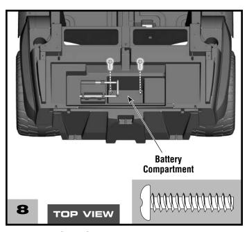
• Insert two 1/4" x 11/4" screws inside of the battery compartment and into the front end of the vehicle. Tighten the screws.
