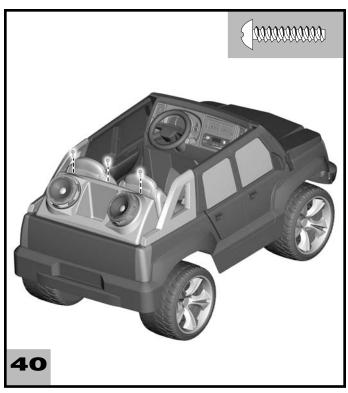
• Insert three #8 x 3/4" screws into the top of the speaker assembly. Tighten the screws.
