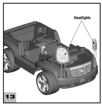
• Fit the headlights (left and right) onto the bumper. **Hint:** Headlights only fit one way. If they do not seem to fit, try the other side.
