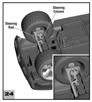
• Insert the curved end of the steering column through the hole in the steering rod.
