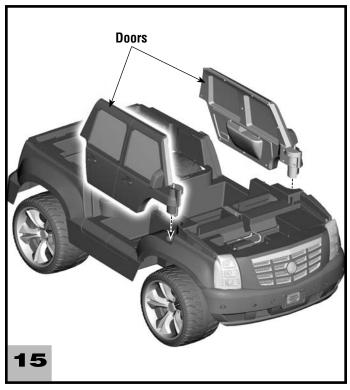
• Fit the door pegs onto the holes near the front end of the vehicle.
