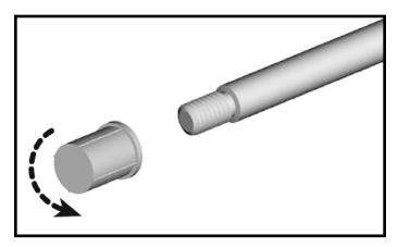
**Note:** Protective caps have been added to the threaded metal parts to prevent damage during shipping. Please remove and throw the caps away.
