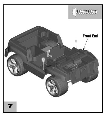
$\bullet$  Insert two #8 x  $^3/^4$  screws through the front end and into the vehicle. Tighten the screws.
