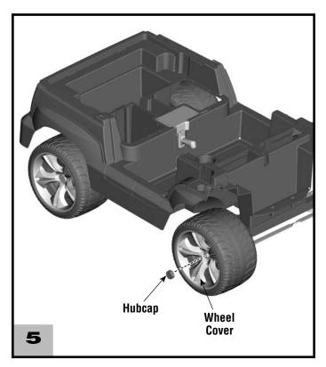
• Align the slot in a hubcap with the rib in the wheel cover. "Snap" a hubcap into the center of each wheel cover.
