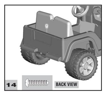
• Insert a #10 x 3/4" screw into the rear edge of the seat and tighten.
