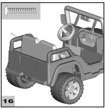
• Insert a #10-32 x 1" screw through the hole in each grab bar and into the seat. Tighten the screw.
