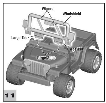
Position the windshield so that the molded detail on the wipers faces the front of the vehicle.
