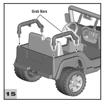
• Fit a grab bar onto each side of the vehicle, as shown.
