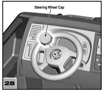
• Insert and "snap" the steering wheel cap into the center of the steering wheel.
