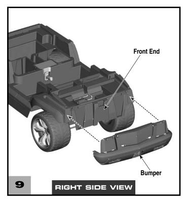
• Fit the bumper onto the front end.
