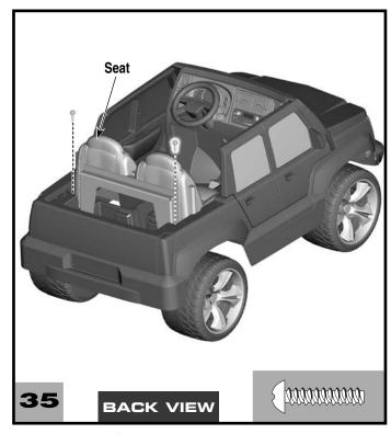
Insert two #8 x <sup>3</sup>/4" screws into the back of the seat. Tighten the screws.
