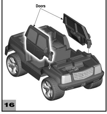
• Fit the door pegs onto the holes near the front end of the vehicle. *Hint:* There is a left and right door. They are designed to be assembled one way.
