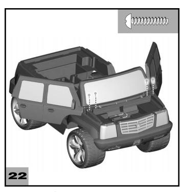
• Insert four #8 x <sup>3</sup>/4" screws into the base of the windshield/dash. Tighten the screws.
