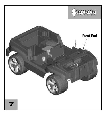
• Insert two #8 x <sup>3</sup>/4" screws through the front end and into the vehicle. Tighten the screws.
