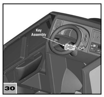
• Insert and "snap" the key assembly into the slot in the dash.
