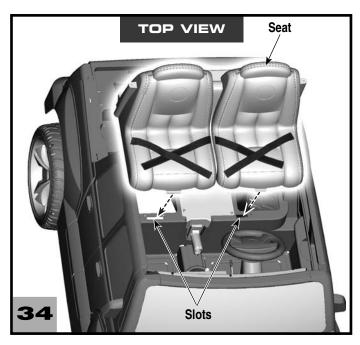
• Insert the two tabs on the front edge of the seat into the slots in the vehicle.
