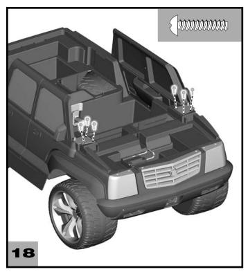
• Insert three #8 x 3/4" screws into each plate and tighten.
