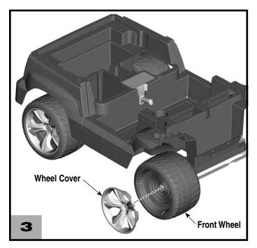
· Fit a wheel cover onto each front wheel.
