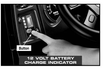
Press the 12 volt battery charge indicator button to check the power level of your battery:
