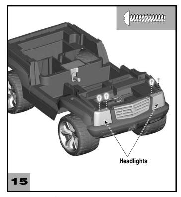
• Insert two #8 x 3/4" screws into the top edge of each headlight. Tighten the screws.
