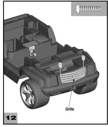
• Insert two #8 x  $^{3/4}$ " screws the top of the grille. Tighten the screws.
