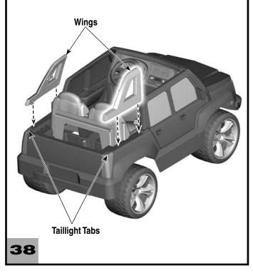
• Fit the wing tabs into the slots in the top edge near the rear of the vehicle.
