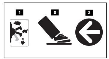
**IMPORTANT!** To avoid damaging the motors and gears, stop the vehicle before shifting from forward to reverse.
