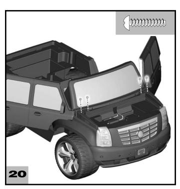
• Insert four #8 x 3/4" screws into the base of the windshield/dash. Tighten the screws.
