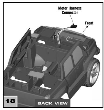
• Position the motor harness connector towards the front of the vehicle and into the battery compartment.
