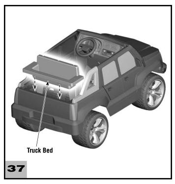
• Position the truck bed over the back end of the vehicle.
