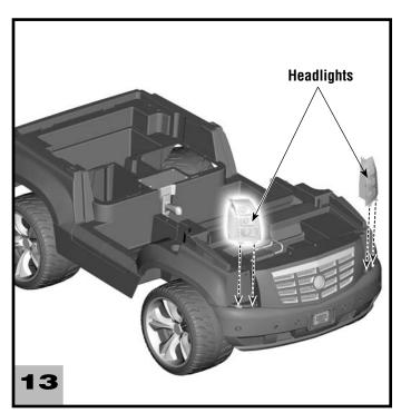
• Fit the headlights (left and right) onto the bumper. **Hint:** Headlights only fit one way. If they do not seem to fit, try the other side.
