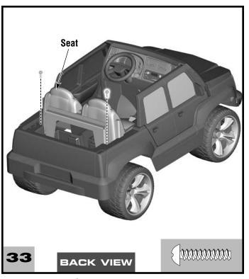
Insert two #8 x 3/4" screws into the back of the seat.
