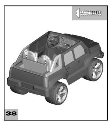
• Insert three #8  $\times$  3/4" screws into the top of the truck bed. Tighten the screws.
