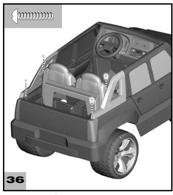
• Insert two #8 x 3/4" screws into each wing. Tighten the screws.
