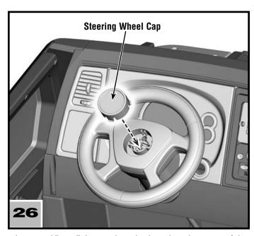
Insert and "snap" the steering wheel cap into the center of the steering wheel.
