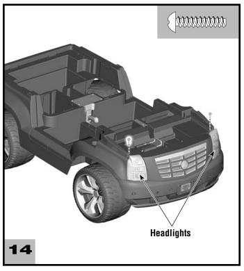
• Insert one #8 x  $^3/^4$  screw into the top edge of each headlight. Tighten the screws.
