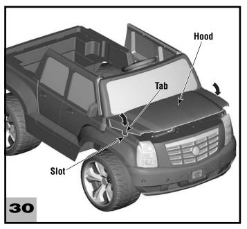
Lower and fit the side tabs on the hood into the slots on each side of the front end of the vehicle.
