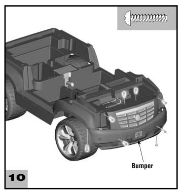
• Insert eight #8 x 3/4" screws into the bumper and tighten.
