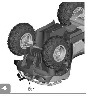
• Grasp the bar on the front end and pull it out and up to properly position the front end.
