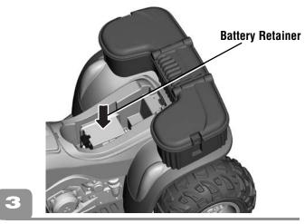
• Carefully lower the battery into the battery compartment. The battery retainer slides over the battery to secure it.
