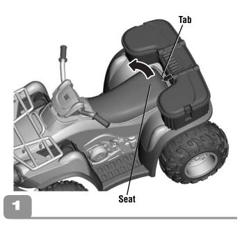
Press the tab on the rear of the seat and lift to remove.
