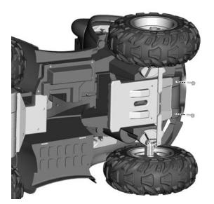
• Insert two #8 x 3/4" screws though the front end and into the base plate. Tighten the screws.
