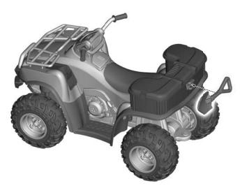
· Attach the shovel onto the rear of the vehicle.
