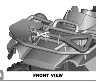
Using safety scissors, cut the plastic cable holding the shovel to the front rack on the vehicle.
