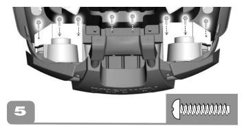
• Now, fit eight more #8 x  $^{3}/_{4}$ " screws into the remaining holes in the front end and tighten them.
