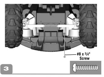
$\bullet$  Fit another #8  $\,$  x  $^3/_4"$  screw through the hole shown in the front end and into the vehicle. Tighten the screw.
