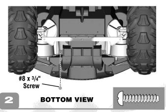
• Fit a #8 x 3/4" screw through the hole shown in the front end and into the vehicle. Tighten the screw.
