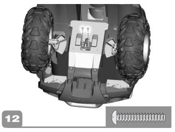
• Insert two #10 x 1" screws into the clip and tighten.
