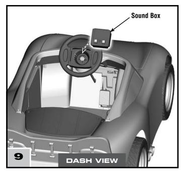
Fit the sound box into the center of the steering wheel. Make sure the buttons on the sound box are downward.
