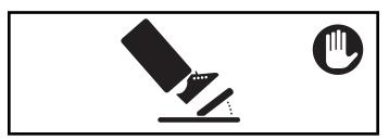
Your vehicle has a patented, electronic braking system that automatically stops the vehicle when your child's foot lifts from the pedal. Make sure your child is comfortable with steering the vehicle and automatically knows how to stop.
