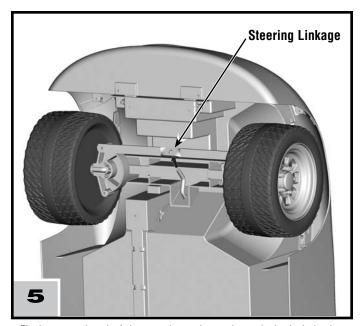
• Fit the curved end of the steering column through the hole in the steering linkage.
