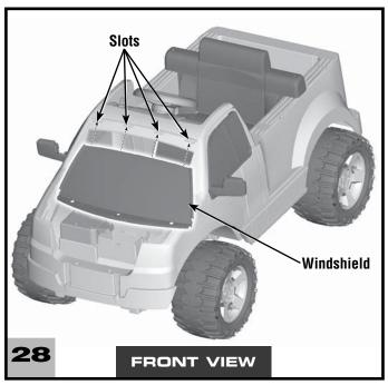
• Insert and "snap" the tabs at the top of the windshield into the slots in the top edge of the vehicle.
