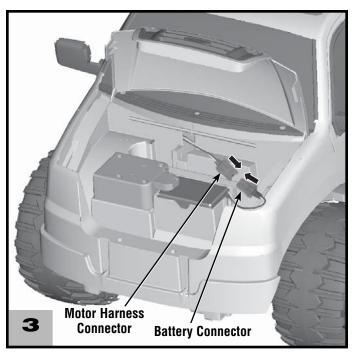
Plug the battery connector into the motor harness connector.
