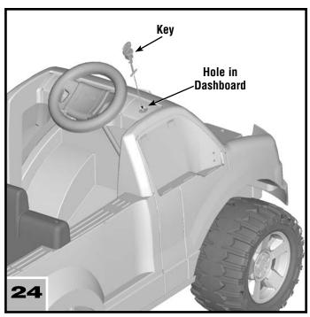
• Insert and "snap" the key into the hole in the dashboard.
