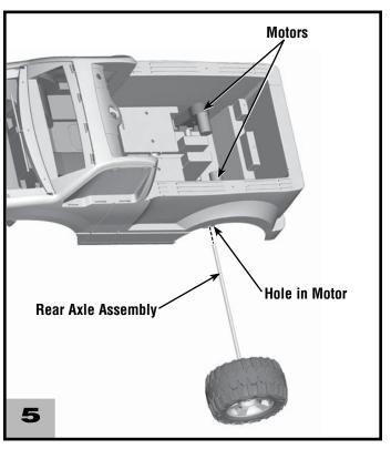
• Slide the rear axle assembly through the hole in one motor, the back end of the vehicle and then out through the other motor.
