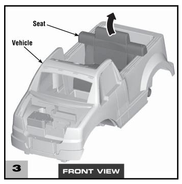
• Rotate the seat back and lift to remove from the vehicle.
