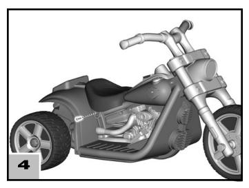
• Replace the screw in the holes on **each side** of the seat and tighten.
