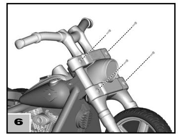
• Insert four screws into the headlight and tighten.
