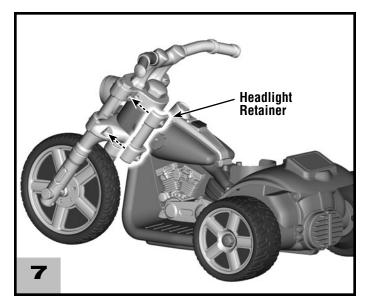
• Fit a headlight retainer to the back of the headlight, as shown.
