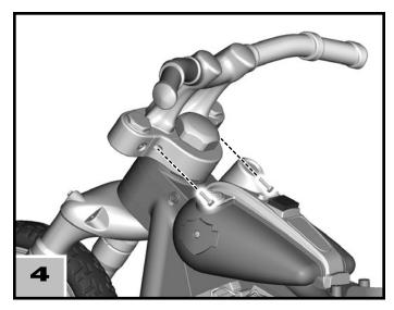
• Insert two screws into the outer holes in the handlebar bracket and tighten.
