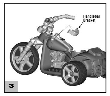
• With the ribbed side down, fit the handlebar bracket onto the back of the front wheel assembly and handlebar, as shown.
